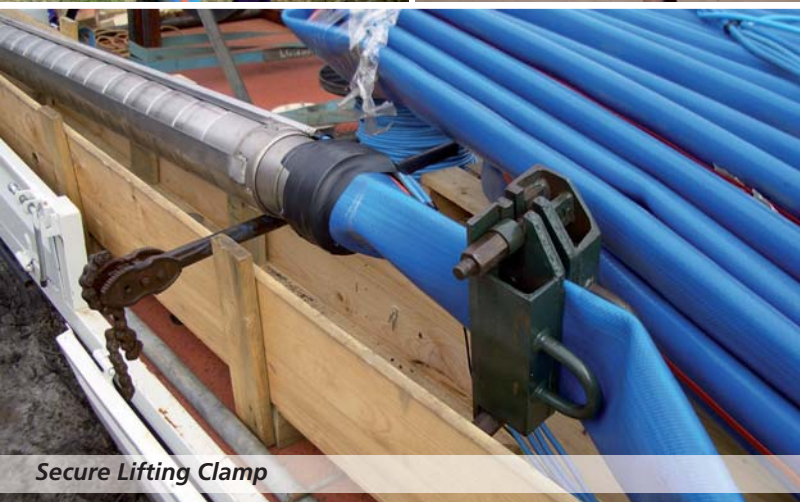
Attach clamp to Hose - ensure power cable is not clamped
